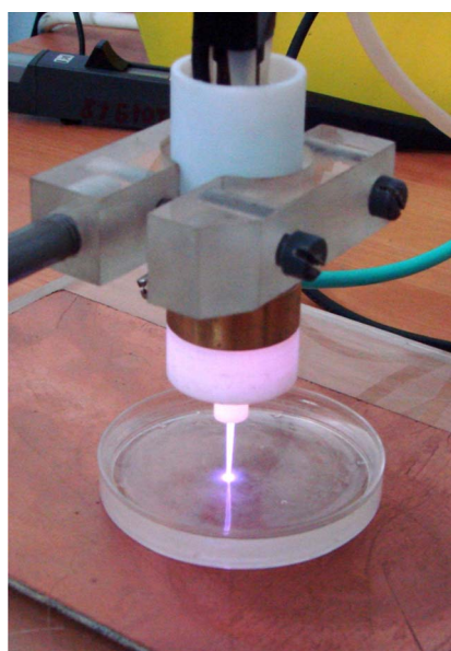
Fig. 3. Final device, generating high-voltage pulsed cold atmospheric plasma jet.
