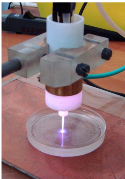
Fig. 1. The final device, generating high-voltage pulsed, cold atmospheric plasma jet.
